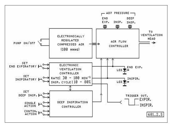
Fig. 3: Functional diagram of the VCM
