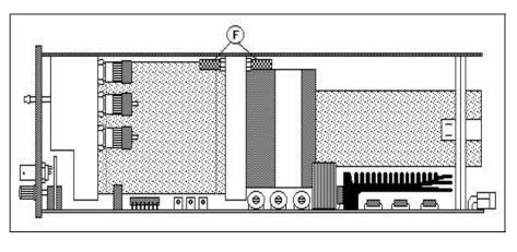
**Fig. 9**: View of module from below. **F**: suction filters. Screw out for cleaning.
