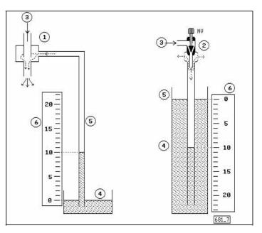
Fig. 8: Preliminary adjustement of the ventilation pessure using a simple water manometer.
