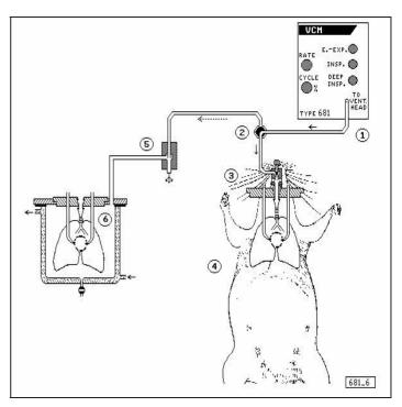
Fig. 7: Positive and negative pressure ventilation with the VCM
