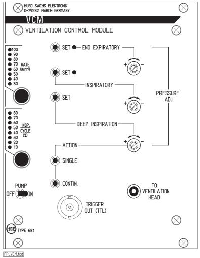
Fig. 2: Front panel
